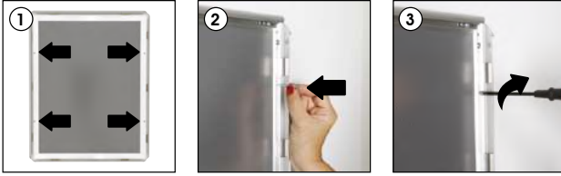
Screw & anchor mounting
